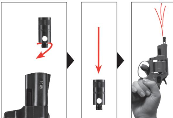
Screw the fireworks adapter into the barrel.
