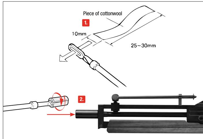
Put the safety on „safe“ and remove the magazine. Prepare a thin rod with a length of approx. 60 cm. Attach a piece of cotton fabric to its end and clean the barrel with some silicone oil.
